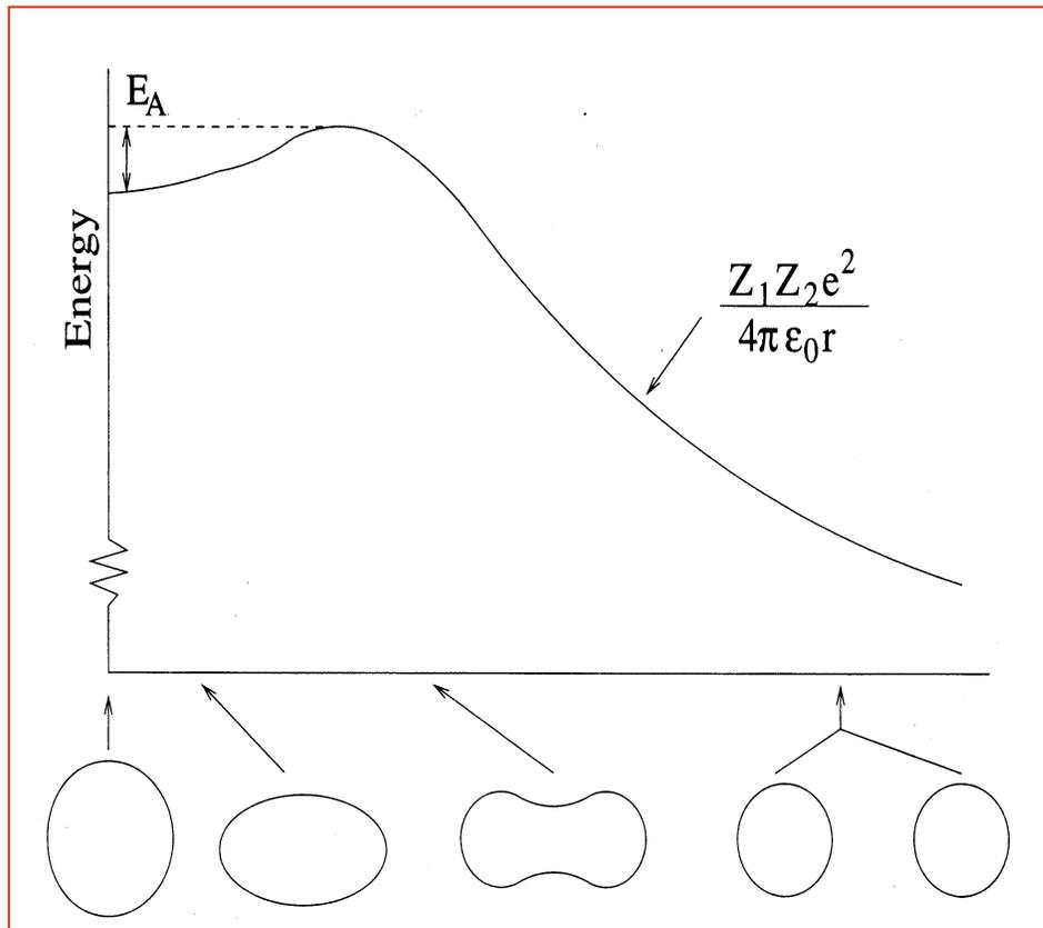
Fission occurs as a result of quantum tunneling through the fission barrier. Normally,  ${}^{235}\text{U}$  decays by alpha emission with only  $\sim 7 \times 10^{-9}$  probability for fission due to a high fission barrier. A thermal neutron is needed to induce the fission by exciting the nucleus, leading to a lower fission barrier thus a larger tunneling probability.
